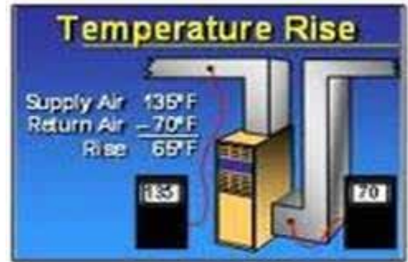
Figure 1: Measuring the supply temperature.
